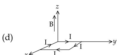
If there is a uniform magnetic field of 0.3 T in the positive  $z$  direction, in which orientations the loop would be in (i) stable equilibrium and (ii) unstable equilibrium ?
