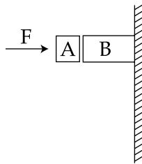
Given in the figure are two blocks A and B of weight 20 N and 100 N, respectively. These are being pressed against a wall by a force F as shown. If the coefficient of friction between the blocks is 0.1 and between block B and the wall is 0.15, the frictional force applied by the wall on block B is :
